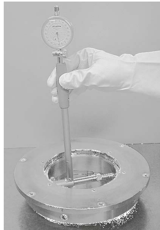
Fig. 1.9 Adjusting the GN Gauge Bore
