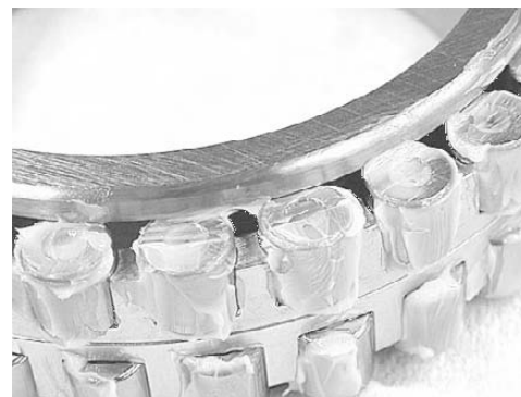
Fig. 1.23 Grease Packed Cylindrical Roller Bearing
