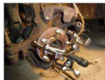
3 Jaw Puller used for removing tyre hub
