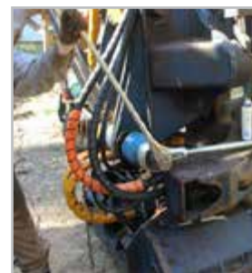
Torque multiplier used for machine nut tightening
