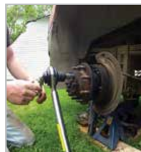
Torque multiplier used for lug nuts
