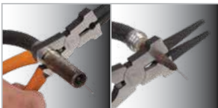
Nozzle removal & installation
