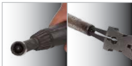
Welding Gun Nozzle filled with weld splatter
