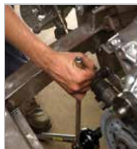
Torque multiplier used in inaccessible areas
