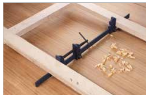
Duo Bar used for internal clamping
