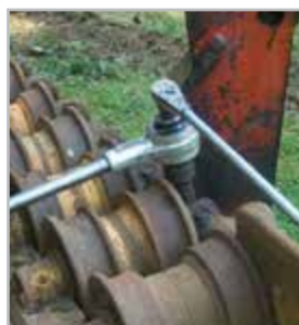
Torque multiplier used on tracks
